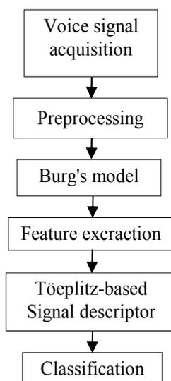
**Fig. 1.** Töeplitz-based signal descriptor in a voice signal recognition system.
